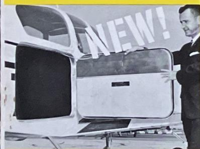
New! Widest cargo door of any light twin is an optional convenience that Baron owners find useful when transporting bulky loads. Measuring 22½ inches high by 38 inches wide, the door can easily accommodate a litter patient when the Baron is used as an ambulance aircraft.
