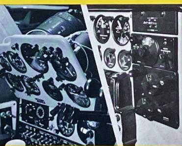
Hinged flight instrument panel speeds service and inspection. Radio and navigation panel is instantly removable, too . . . a time-saving convenience for owners wanting to service or add to their nav/comm equipment.
