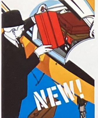
**There's even more room** for baggage in the Baron nose compartment, now that all radio equipment can be accommodated forward in the new longer nose cone. Five or six pieces, totalling up to 270 pounds, can be carried.
