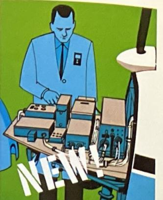
**Tough fiberglass nose shell** is easily and quickly removable, giving unobstructed access to the bench-height radio equipment deck as well as the 50,000 BTU heating plant . . . a time-saving advantage when servicing or adding new equipment.
